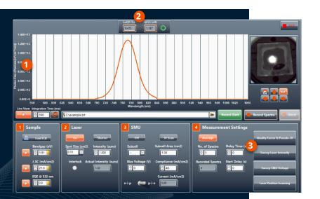
Absolute photon flux measurement Records single or multiple EL/PL spectra for pre-set laser intensity and voltage bias
