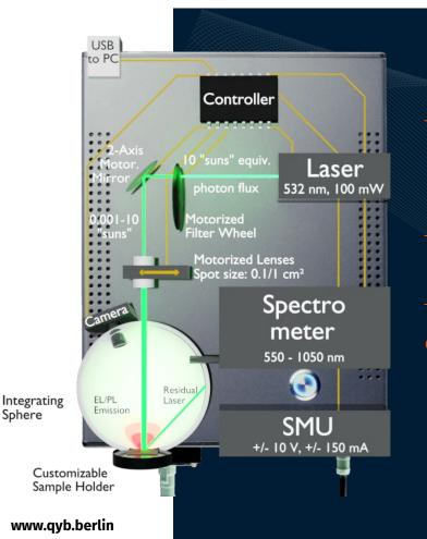
Swift quantification of **Absolute Photon Fluxes** from electro- and photoluminescence (**EL & PL**) of semiconductor thin films & devices
